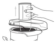
5. Place fingers under the rim of the stainless steel blade and filtering basket and lift out – figure 11. **Important:** Juicing blades are very sharp, handle juicing filter basket with care when removing, replacing and cleaning.
